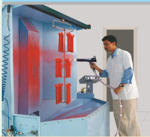
The axial entry cyclone with Rotary Vane technology makes this recovery unit most suitable for fast, multi colour powder coating.
