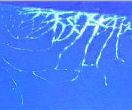
Cracks clearly visible after fluorescent spray
