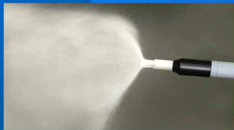
NORMAL GUN WITH EXTERNAL SIEVED POWDER -ALTERED CLOUD PATTERN
