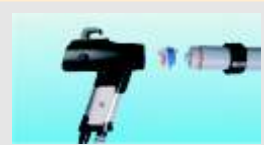
replace the power cartridge
